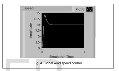
The tunnel wind speed is shown in the figure 4,here the set point is achieved after the overshoot due to the proportional action in the PID controller used, by the same way the model balancing is controlled and achieved as shown in the figure 5.
