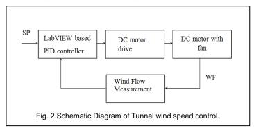
During testing the wind speed in the tunnel changes in accordance with the geometry of the test model and the position of the test model, but the speed of the wind is to be constant for the good test results. To maintain the wind in the constant speed, the current speed of the wind is measured in and around the test model and is fed back to the controller to maintain the constant speed.
